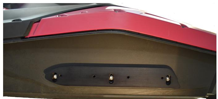
Install left side RIVA sponson blade onto billet backing plate using 4 of the supplied shorter bolts & washers.
